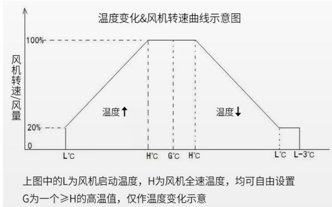
In the figure above,  $L$  is the starting temperature of the fan, and  $H$  is the temperature of the fan at full speed, which can be set freely.
